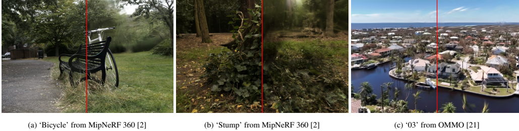
Figure 4: Effect of the noise term ( \epsilon ) – We visualize our reconstruction with (left half) and without (right half) the noise term in (7). The noise terms are essential to explore the full scene extent.
